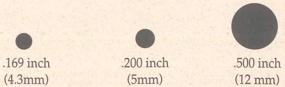
Core diameter of the wood sample is determined by the inside diameter of the opening at the threaded end of the bit. For general forestry use, .169" is commonly used, .200" is used for wood preserving testing and .500" is used for large amounts of wood for quantitative analysis.
