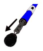
B. Remove the borer auger (bit) from the handle along with the extractor
