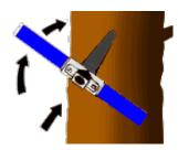
The borer is now ready for use.When screwing the borer into the tree, consider the following: Do not use force starting when the penetration. It may cause damage to your borer and small chips may
