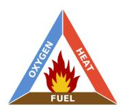
Here are diagrams of the Fire Triangle and the Fire Behavior Triangle. Notice that the one element common to both triangles and the one humans can most directly influence is Fuel.
