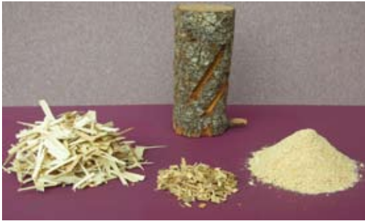
Small-diameter wood is chopped up to make particleboard and other reconstituted products.
